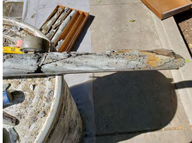
PHOTO 2.1-2: Typical Rock Core
