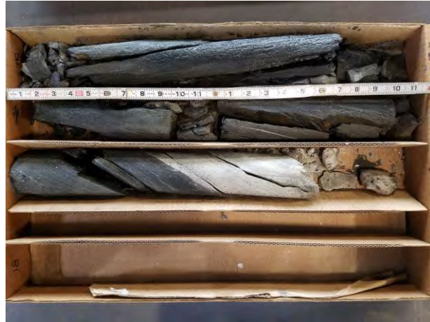
PHOTO 2.5-2: Core from Boring 1-B2
